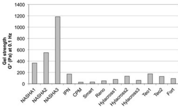
**Figure 6.** Gel strength measured as  $G^*$ , the total resistance to deformation, for the investigated hyaluronic acid (HA) filler products. The products are ordered according to the declared HA concentration in the products.
