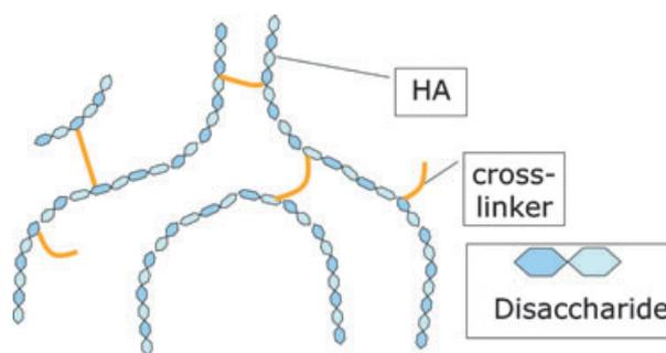
**Figure 5.** Illustration of cross-linkers bound to HA chains. The cross-linker can bind to both ends, creating a cross-link, or bind to only one end, modifying the HA without contributing to gel strength.
