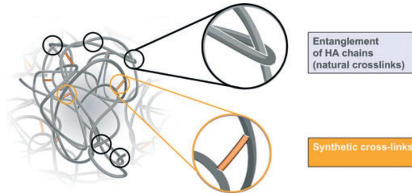
**Figure 1.** Illustration of synthetic and natural cross-links.
