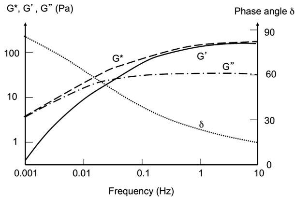
**Figure 2.** Frequency dependency of the viscoelastic properties of a polymer solution.
