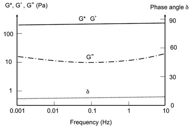
**Figure 3.** Frequency dependency of the viscoelastic properties of a polymer gel.
